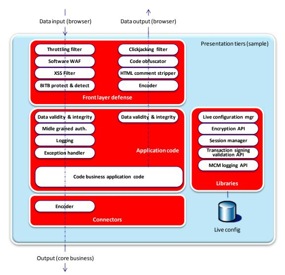
Figure 18 - Application security hardening sample
