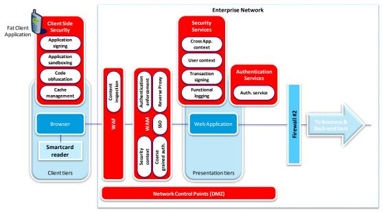
Figure 8 - Mobile security Architecture reference
