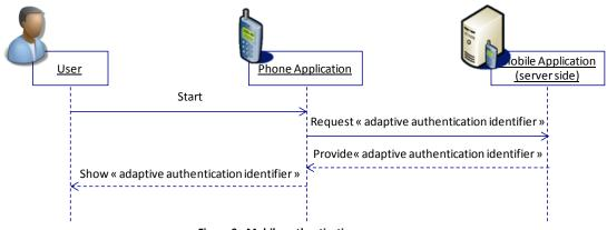
Figure 9 - Mobile authentication process
